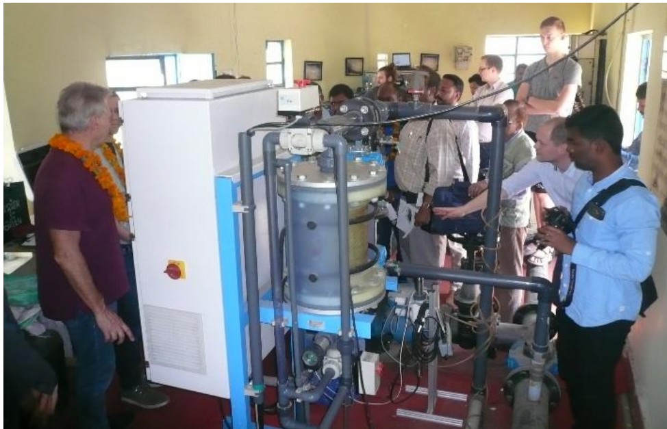
Figure 3. A medium-capacity inline-electrolysis pilot plant is demonstrated to participants at a training course at RBF well No. 18 in Haridwar (photo: HTWD).
